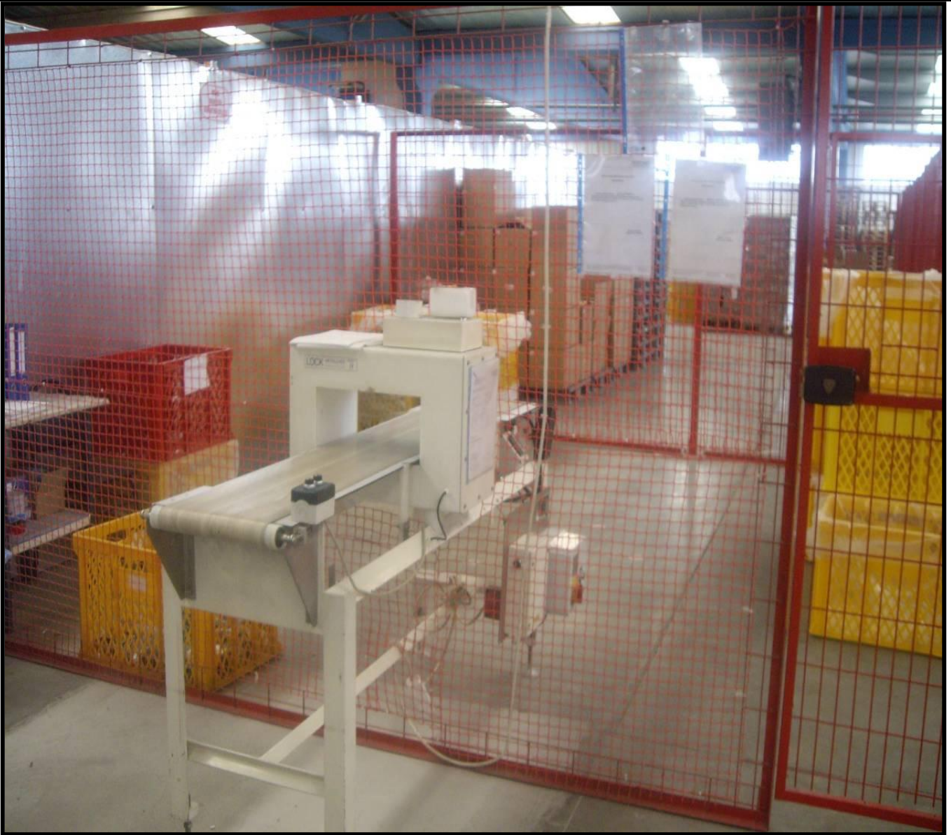
Conveyor belt metal detector well positioned into a secure isolation area
