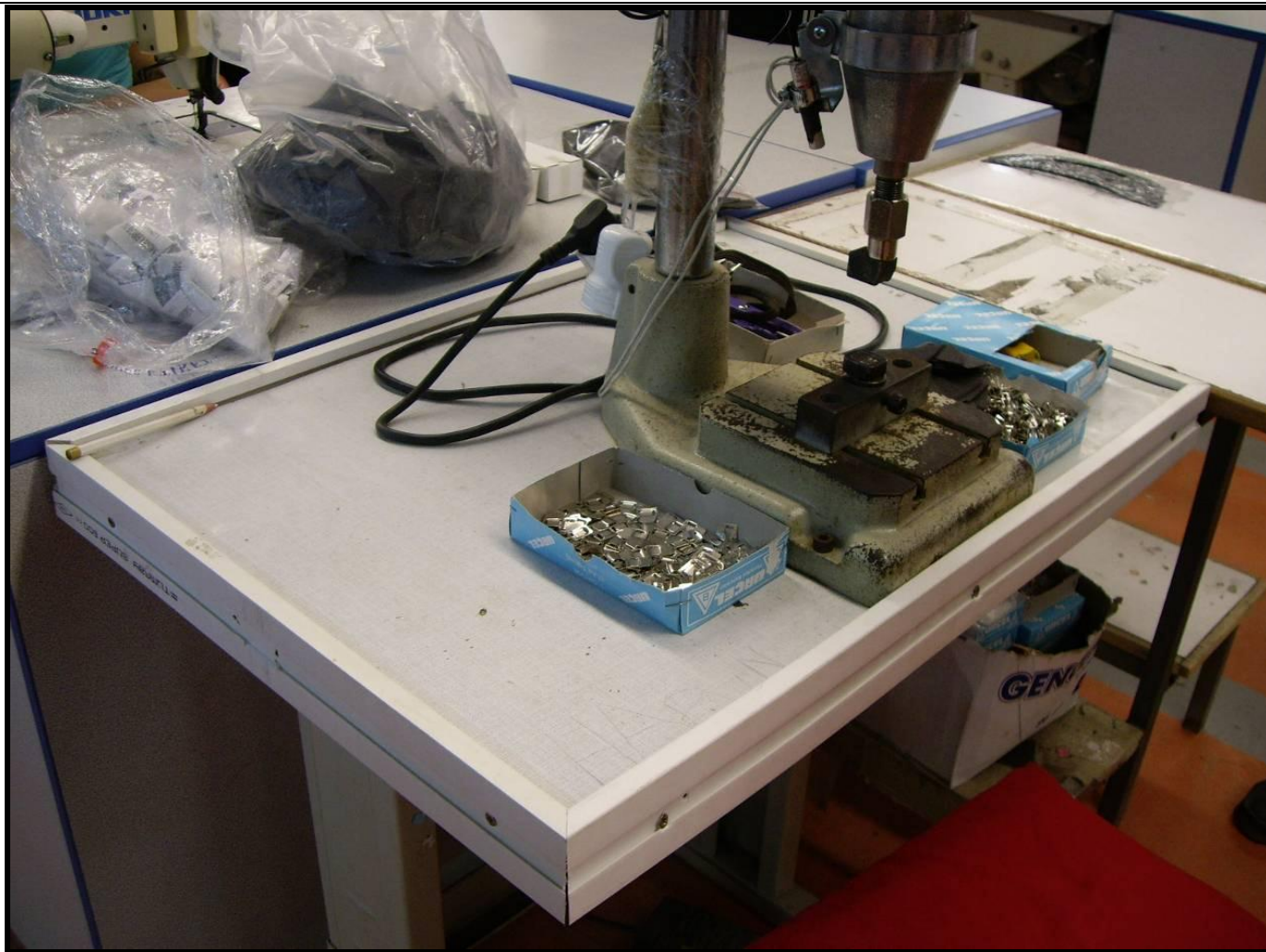
Lip around work bench for containing small metal trims
